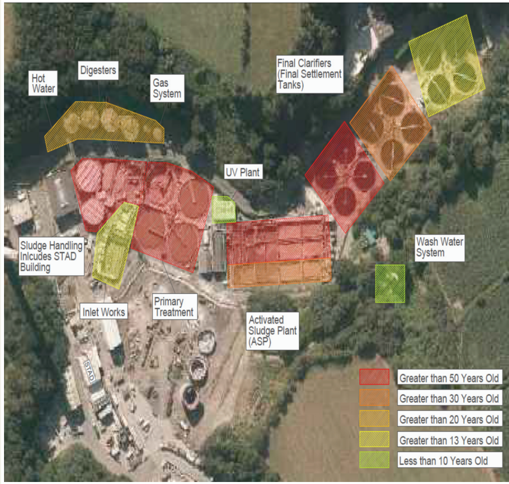
FIGURE 69 – AGEING SEWAGE TREATMENT WORKS
